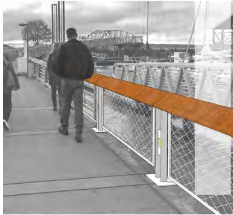
Alternative 1. New posts, crimped edge metal mesh panels and an updated top rail reminiscent of the existing Portwalk railing
